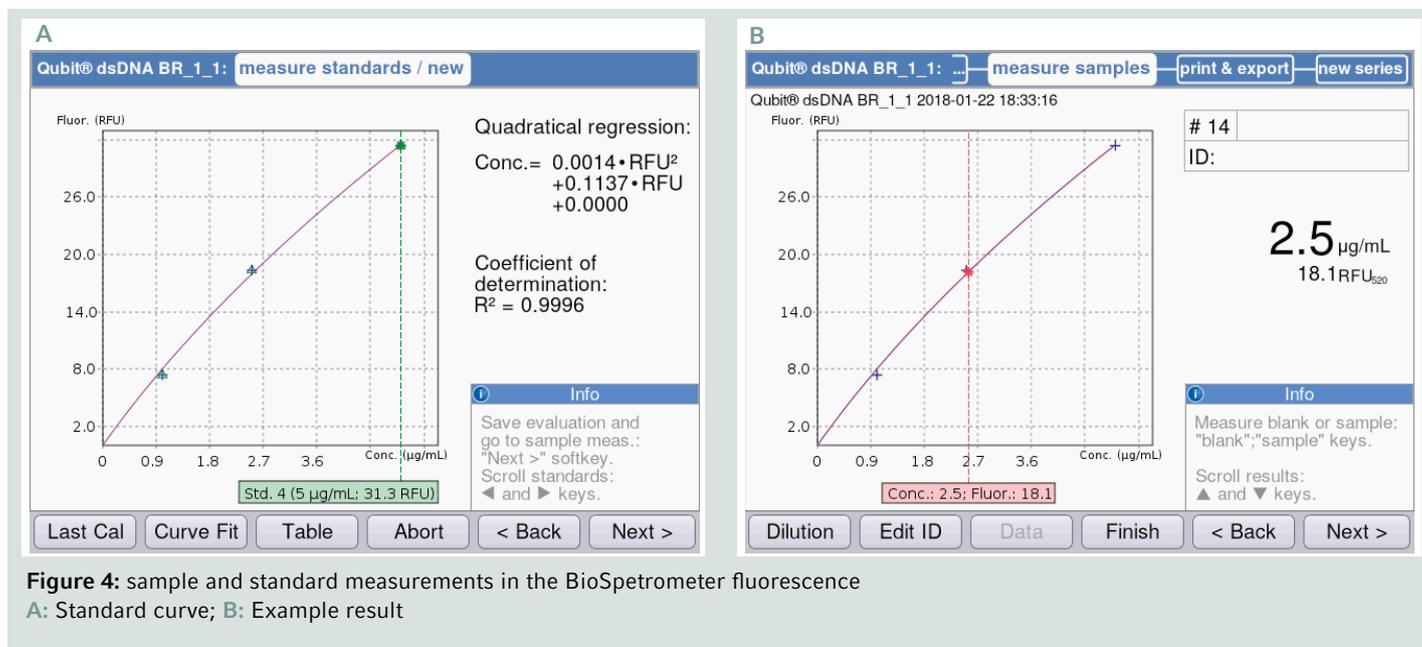
**Figure 4:** sample and standard measurements in the BioSpectrometer fluorescence
